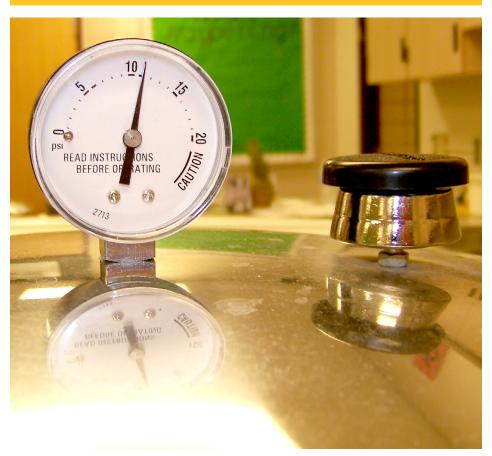
Correct pressure is important when canning low-acid foods such as meats and vegetables. As water boils in a canner, it expands to steam and pressurizes the canner. Pressure in the canner affects the temperature at which water boils. At sea level and 0 pounds on a pressure gauge (0 psig), water boils at 212°F. As the canner heats and pressure builds, the boiling point of water increases and the temperature of circulating steam and water also increases.
