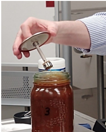
A wireless data recorder is placed inside a filled jar of food to monitor temperature and the cold spot.
