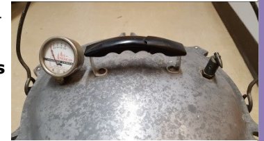
Older All American Canner. The petcock on the right can be replaced with a weighted gauge. Contact Wisconsin Aluminum Foundry .
